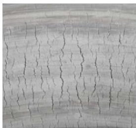
Fig 1 Heavy heat checking
